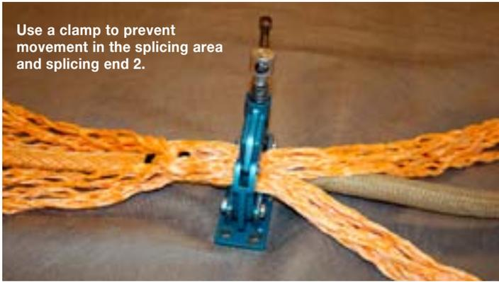
Use a clamp to prevent movement in the splicing area and splicing end 2.
