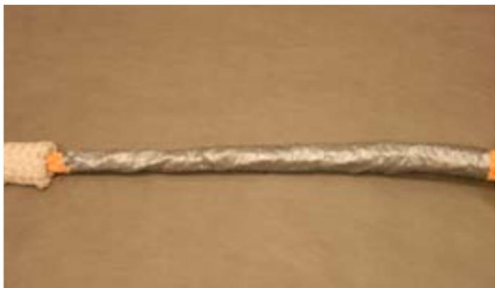
Cover the splicing end with tape to make it easier to put a new section of protective jacket in place.
