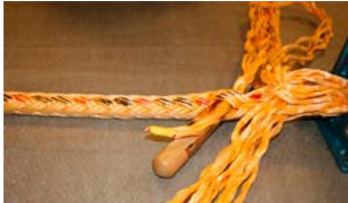
Take the spike under the first two strands and pull the first set of four strands over one red and under two black.
